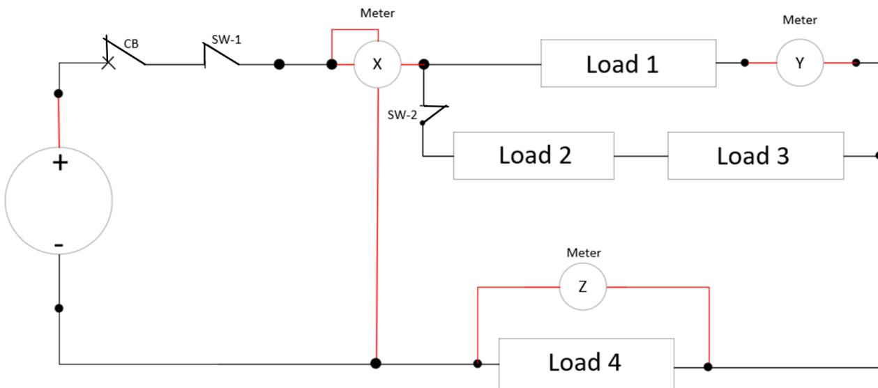
For the circuit shown above, you have taken some measurements with **switch one and two closed** and recorded the following:
