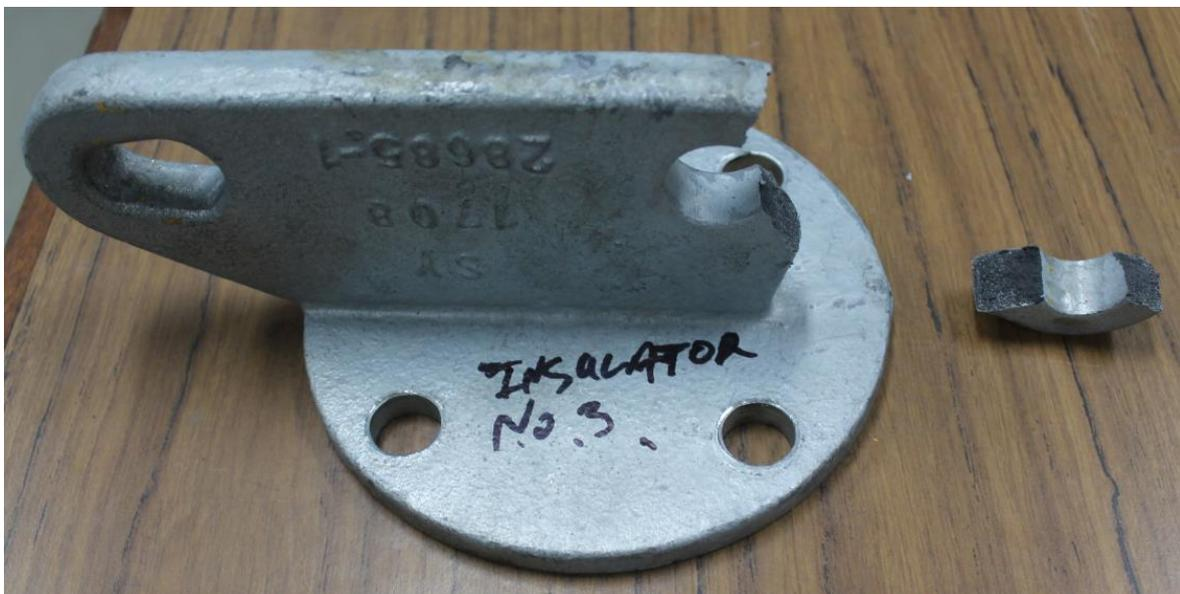
**Figure 8: Image of a failed bracket after the mechanical failing load test**
