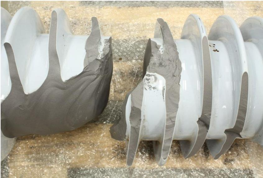
Figure 2: Close-up view of the two main sections of the failed insulator
