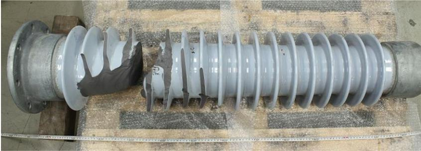
Figure 1: Overall view of the two main sections of the failed insulator
