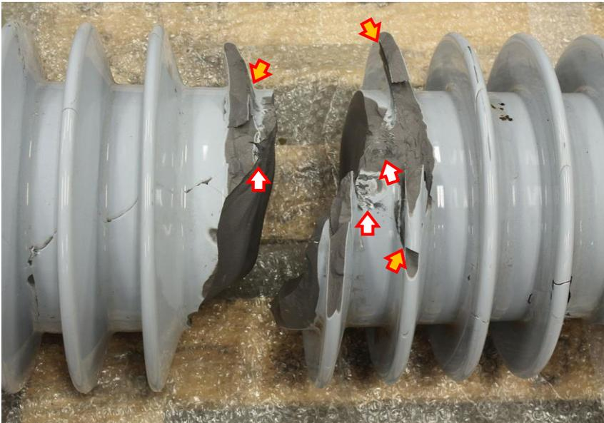
Figure 3: Views of the fractured region of partially reconstructed insulator
